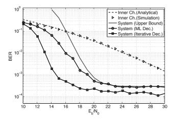
Fig. 3. BER performance comparison for the proposed decoding scheme with standard decoder, number of sensors: 4, frame length: 256, Observation accuracy is modeled as a BSC channel with crossover probability: 0.01.
