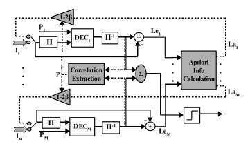
Fig. 2. Decoder structure based on multiple turbo decoder.
