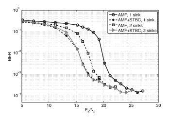
Fig. 4. BER performance of the proposed coding scheme with one and two sinks operating in amplify and forward mode with and without DSTBC.
