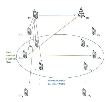
Fig. 1. System model:coexistence of a single primary source-destination link and multiple secondary links. The blue circle encompasses the SUs with acceptable credit history that are candidates for cooperative relaying.
