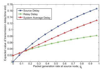
Fig. 3. Average packet transmission delay of system versus packet generation rate at source node.
