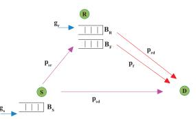
Fig. 1. System model for the proposed relay network, where S, R and D represent source, relay and destination nodes, respectively.
