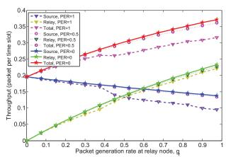
Fig. 4. Average throughput of system versus packet generation rate at relay node for different packet error rates.
