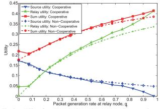
Fig. 2. Utility of source and relay nodes versus packet generation rate at relay node for cooperative and non-cooperative games.
