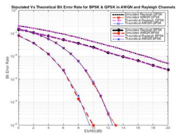
Figure 4: Performance of DS-CDMA BPSK and QPSK modulation in AWGN and Rayleigh environment
