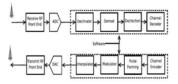
Figure 1: Block diagram of a typical software defined radio system
